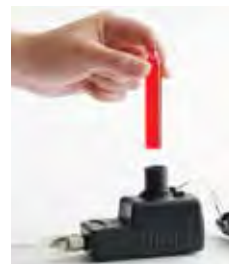
Place in Water Quality Colorimeter and read your results.
