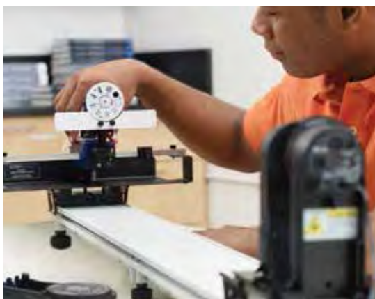
The light sensor combines with the rotary motion sensor for the diffraction of light experiment.
