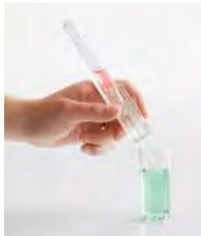
In this titration for Alkalinity, color initially changes to pink.
